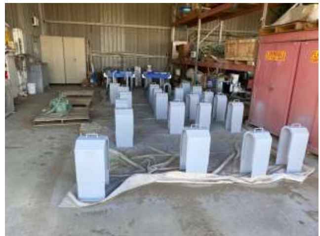
Painting Coupler Safety Guards for Horizontal Pumps
